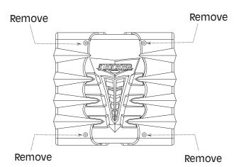
Now that you are ready to mount your amplifier, use the supplied 3mm allen wrench to remove the amplifier EndKap. This will give you access to the mounting holes in the amplifier and all wiring connections.
